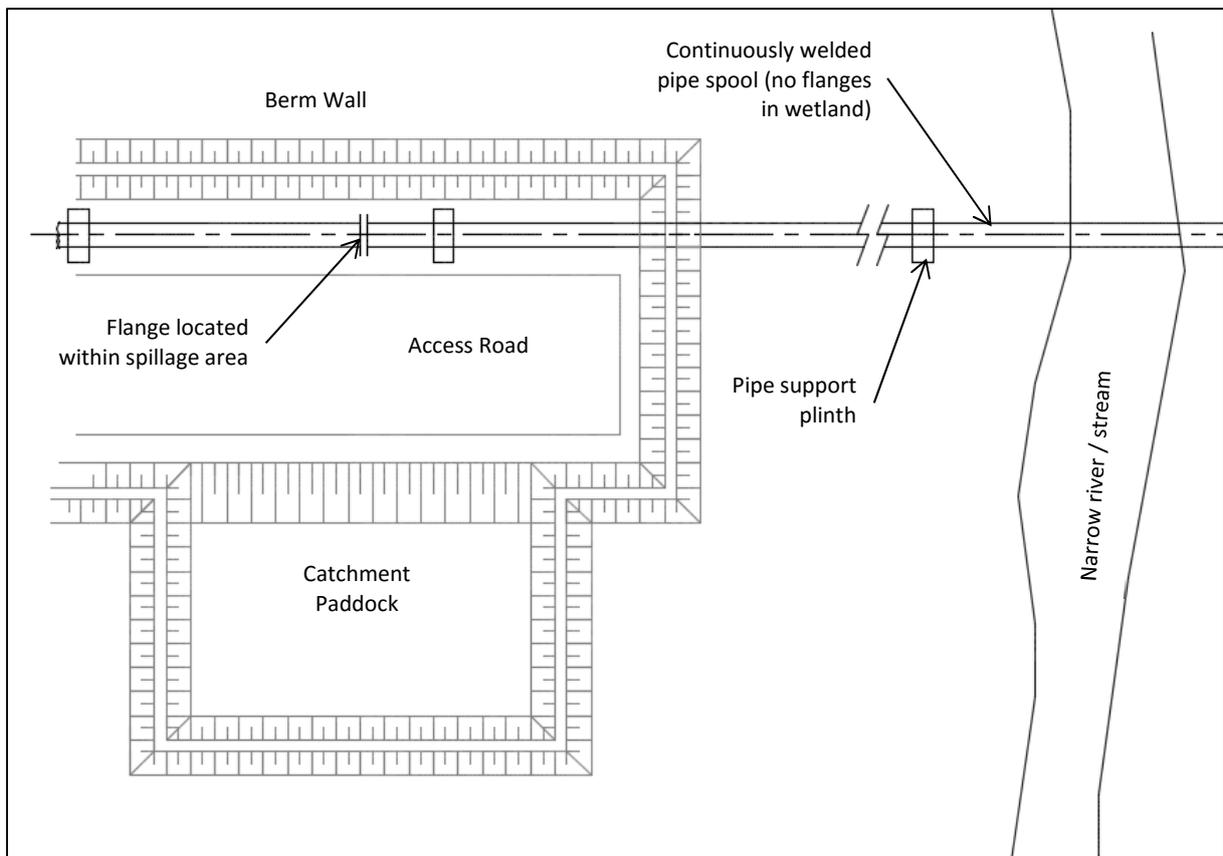
Figure 3: Class 2 River Crossing Spillage Paddock Plan View
