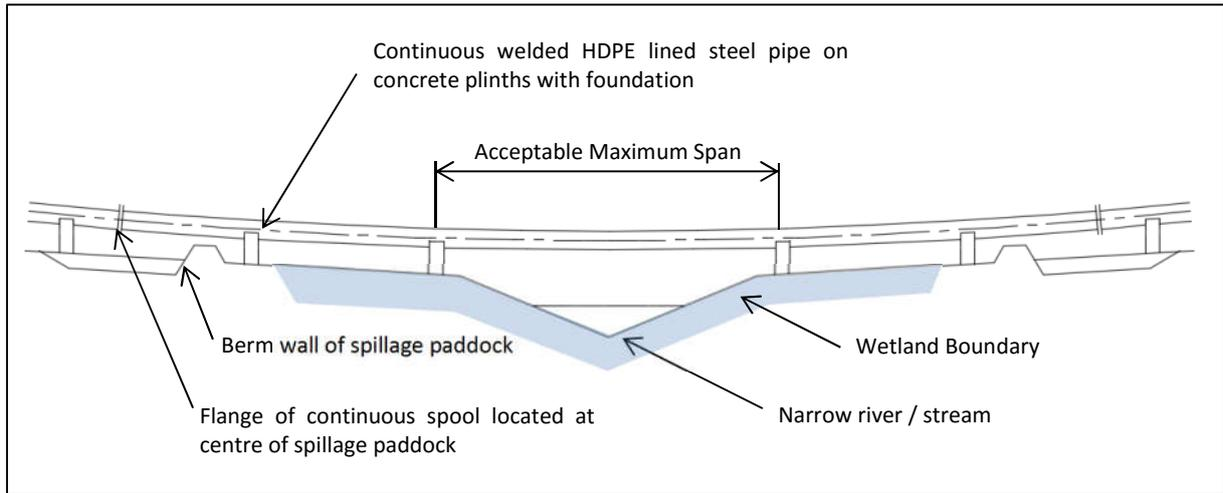
Figure 2: Class 2 River Crossing Cross Section
